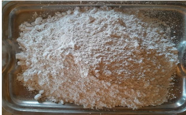
Fig. 4: Cement Kiln Dust (CKD)
