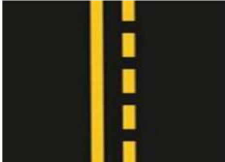
Figure 14. Broken and solid yellow lines DPWH Manual, 2012.
